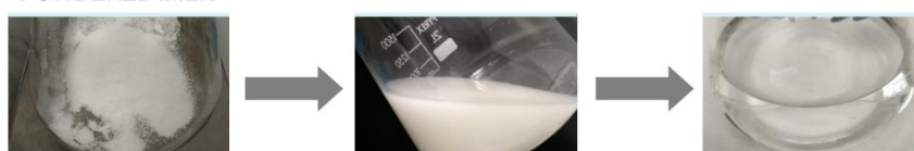
Figure 7: Examples of digestion of shrimps, clams, and powdered milk with the developed sample preparation.
