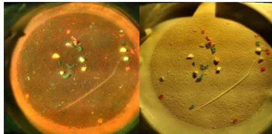
Photographs of a filter stained with NR containing MPs of different colors and polymers.
