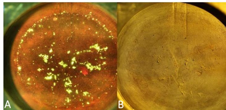
**Figure 3:** Blue light images of nine blank mussels spiked with twenty LDPE particles in the size range of 180-355  $\mu\text{m}$ .
